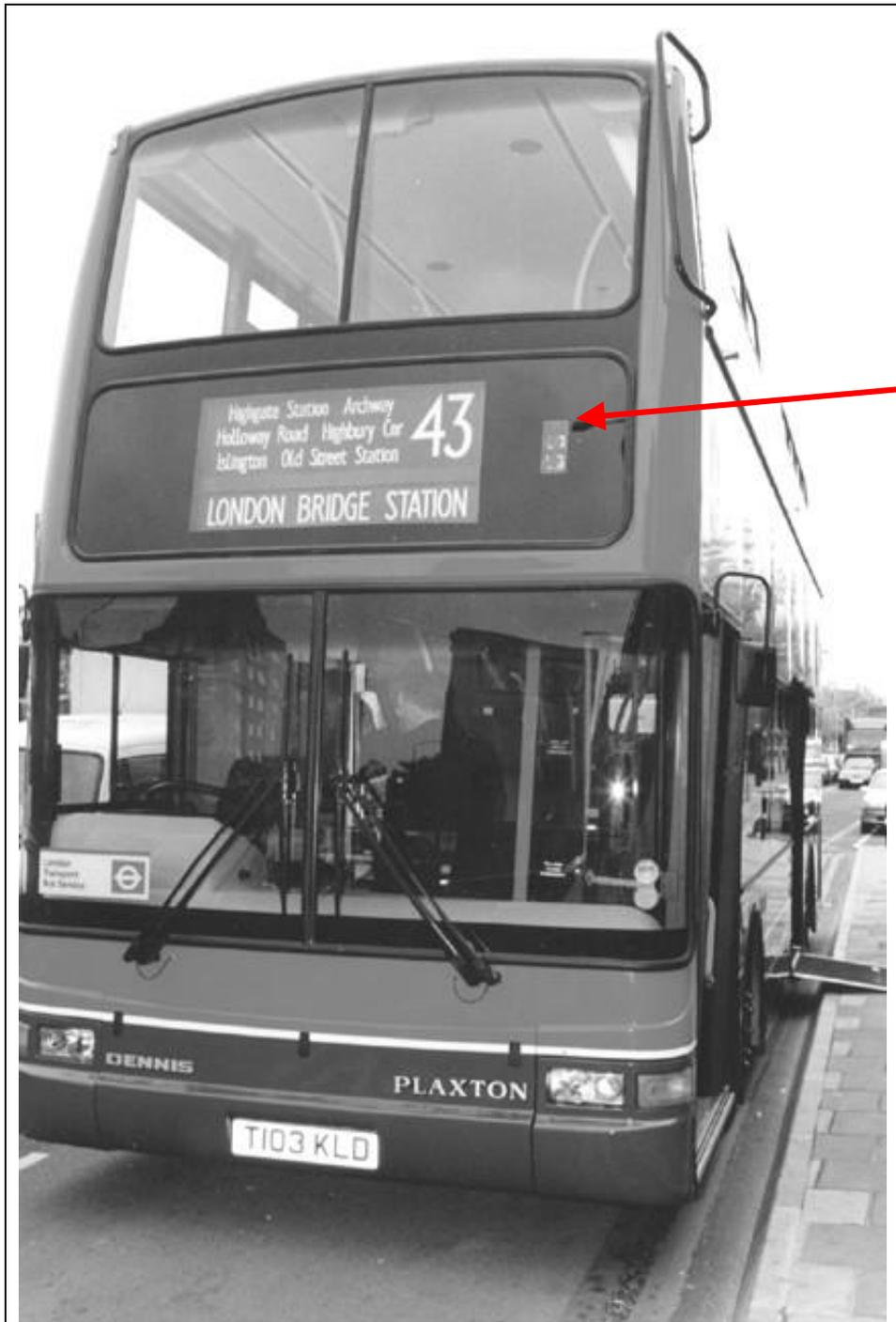
Photograph 8: Bus-mounted bus lane enforcement camera
